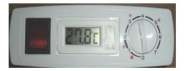
Setting the temperature control to the coldest setting may causethe evaporator coil to freeze and ice up. This will eventually result in a warmer cabinet temperature.
